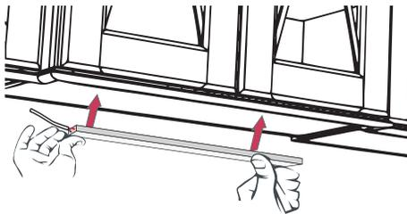
1. Center the fixture in the mounting space. Measure 1/2" from each end of fixture for mounting clip placement. Use screws to secure clip to mounting surface.
