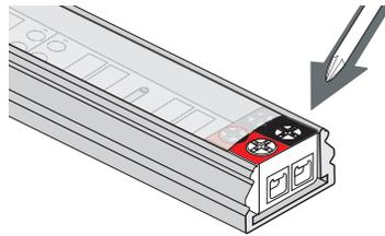
2. Leave frosted lens on the fixture. Use #1 Phillips to loosen the 2 outer terminal screws on the 8MM-EZ Connector. **NOTE: DO NOT loosen the two inner terminal screws.**
