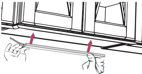
1. Center the fixture in the mounting space. Measure 1/2" from each end of fixture for mounting clip placement. Use screws to secure clip to mounting surface. **NOTE: When installing a fixture 30" and longer, center the third mounting clip between these.**
