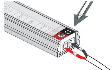
2. Insert stripped wires from power supply or receiver into outer terminals, Red wire to (WW+) side marked in red, Black wire to (CW-) side of tape marked in black; tighten screws.
