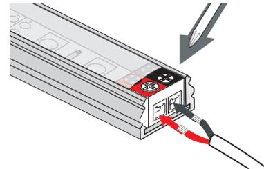
2. Insert stripped wires from power supply or receiver into outer terminals, Red wire to (+ or DC12V) side marked in red, Black wire to (- or GND) side of tape marked in black; tighten screws.
