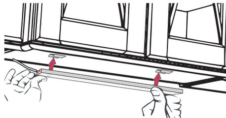
2. Snap fixture into mounting clips.
