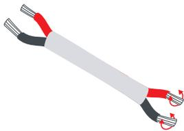
1. Use wire strippers to strip wire 1/4", then twist ends. **NOTE: wires may be folded over after being twisted, but it is not required.**
