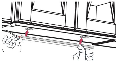
2. Snap fixture into mounting clips.
